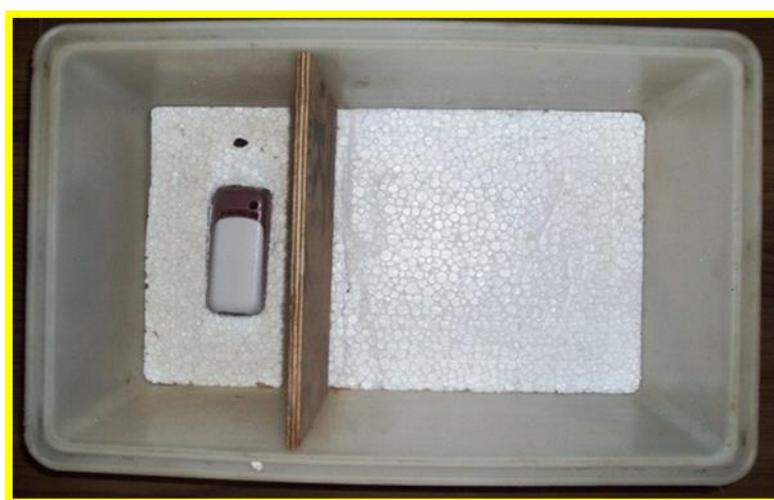
**Fig I:- Photograph Showing Arrangement Of Mobile Phone In Cage.**
